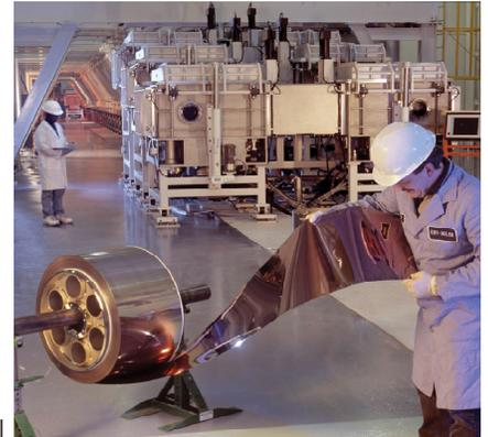
*Uni Solar*® brand solar laminates start with a .005 inch (0.13 mm) stainless steel substrate.
