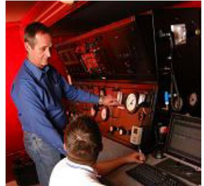
Quarter-inch lines run to an analyzer system that senses chamber depth and carbon monoxide levels and is monitored by the chamber attendant.
