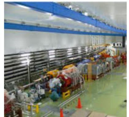
The beam line to extract and transport beams from accelerator to the target. It is constructed from more than 100 electromagnets. More than 10,000 Swagelok tube fittings are used in the facility (J-PARC).
