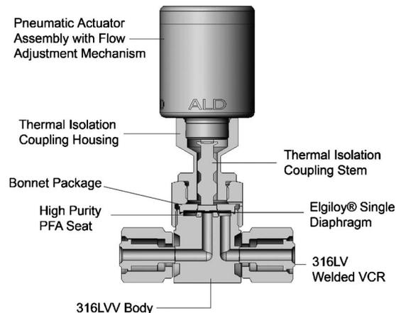
FIG. 2. Swagelok<sup>®</sup> ALD valve wetted and nonwetted materials of construction.
