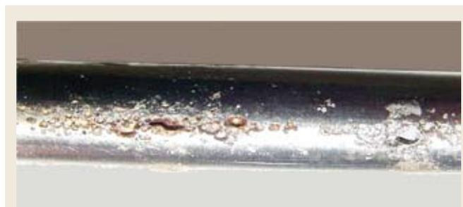
**Fig. 1.** Pitting corrosion of 316 stainless steel tubing.
